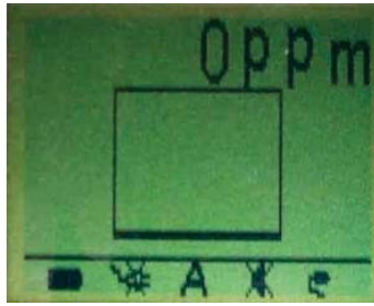
Figure 4: Completion of Zero routine
